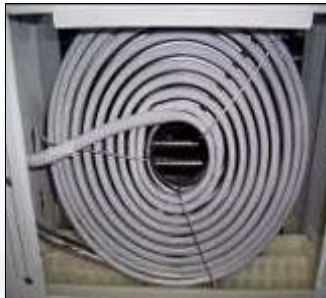
Multiple layered Evaporation Coils
